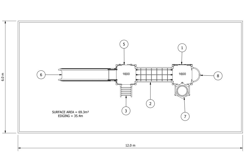
ITEM PS VERTICAL R 1 2 PS Cable Rope 3 PS Ladder 1600 4 PS Steel Pcoat PS Vertical Rock 5 PS Slide Big Dip 6 PS Climbing Rir 7 8 PS Sliding Pole
