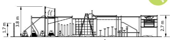
TOTAL AREA =  $376m^2$ RUBBER PATH AREA =  $87.4m^2$  $MULCH AREA = 288.6m^2$ EDGE PERIMETER = 75.5m
